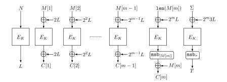
Fig. 2. OCB2 for the case of empty AD.
